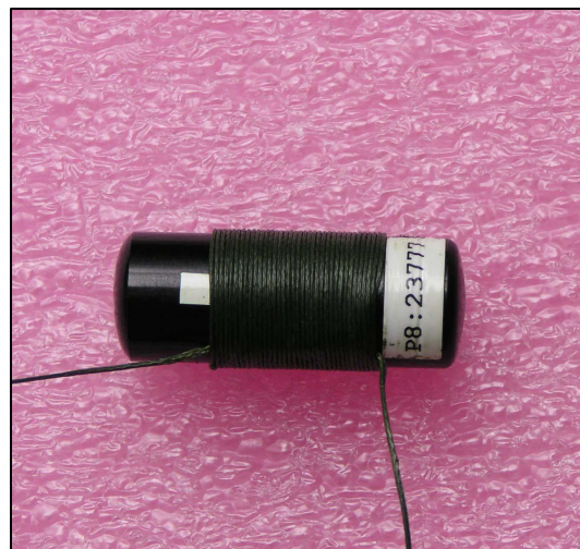
260 Figure 2. A Vemco V9-2H tag after attaching the spiderwire line as a harness. Photo courtesy of MoE.
